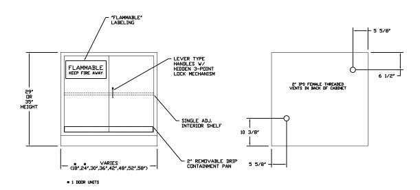
TYP. SECTION FLAMMABLE CABINET REAR VIEW
