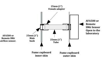
The monitor or sensor must be positioned where it can"see" the room pressure of the laboratory. The back connection spigot of the monitor or sensor will accept the 25mm (1") hose which should be connected to the inner chamber of the Fume Cupboard. The ideal position for the hose connection is 100mm (4") back from the sash and 100mm (4") higher than the normal sash opening height.
